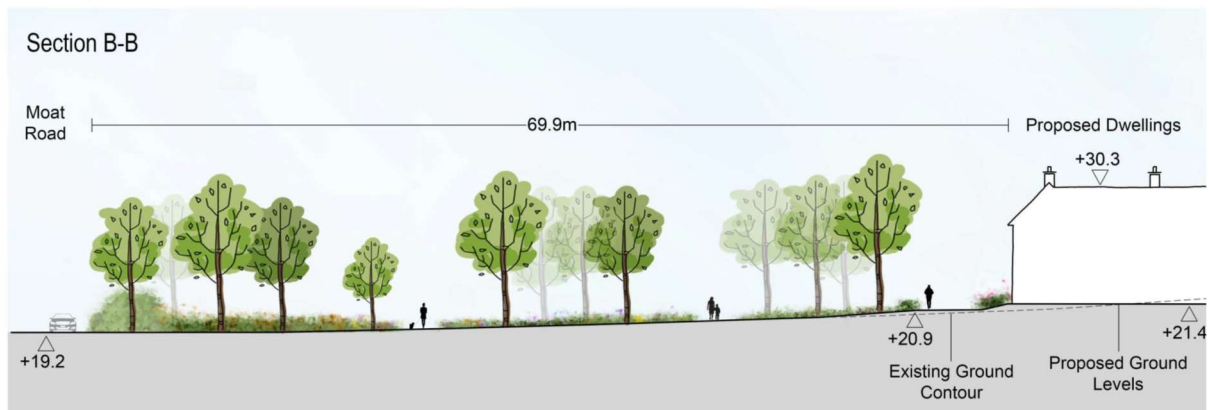
Fig.4 Section B-B (pg. 33 of DAS) showing building set back from Moat Road and landscape corridor to southeast area of the site.
