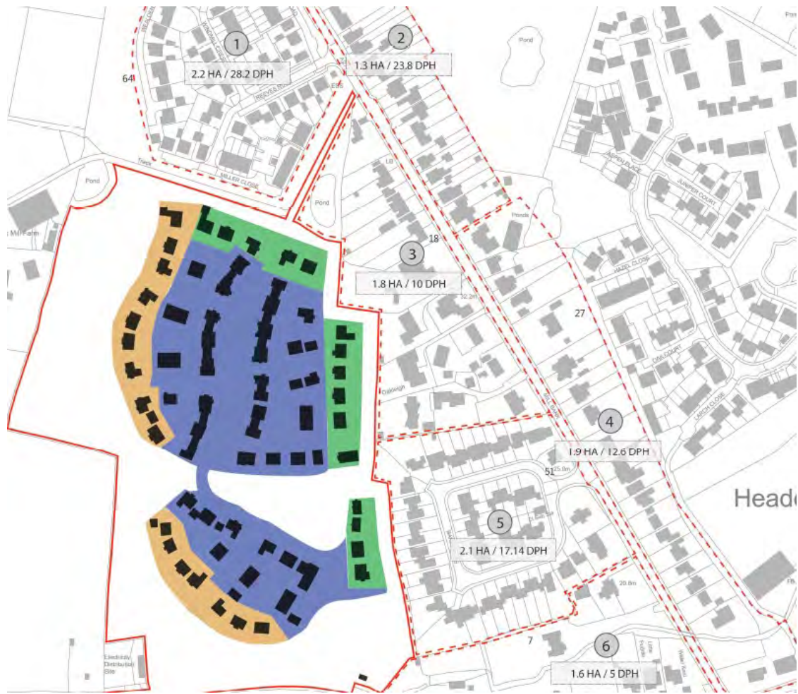
Image EDP 6.1: Proposed updated Character Areas/Densities Plan. Orange areas (Rural Development Edge) are proposed at 21.9dph, blue areas (Main Street and Core) at 33.3dph and green areas (Settlement Edge) at 33.8dph. Surrounding densities are shown for information.
