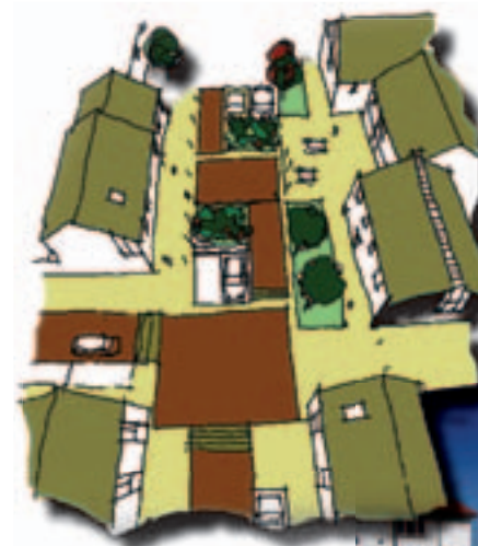
Diagram showing arrangement of planting and car parking in a homezone street. Paving is used to mark out play areas from the carriageway.
