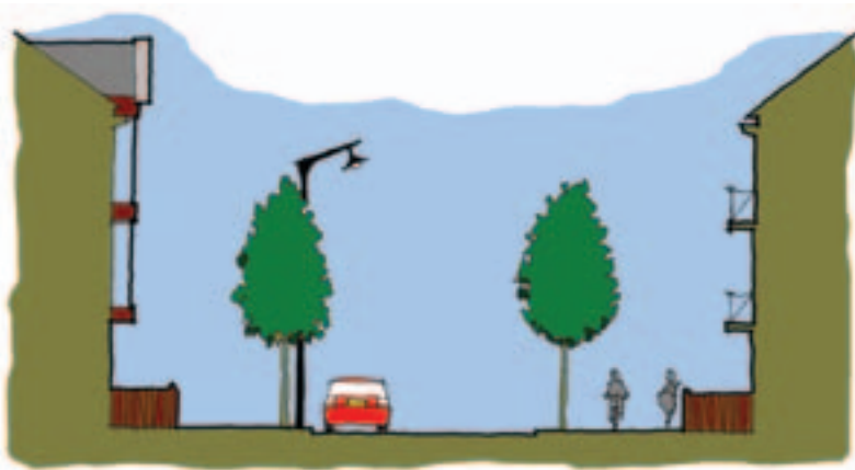
Diagram showing a Local distributor road with scope for an avenue of tree planting, cycle way and footway combined.
