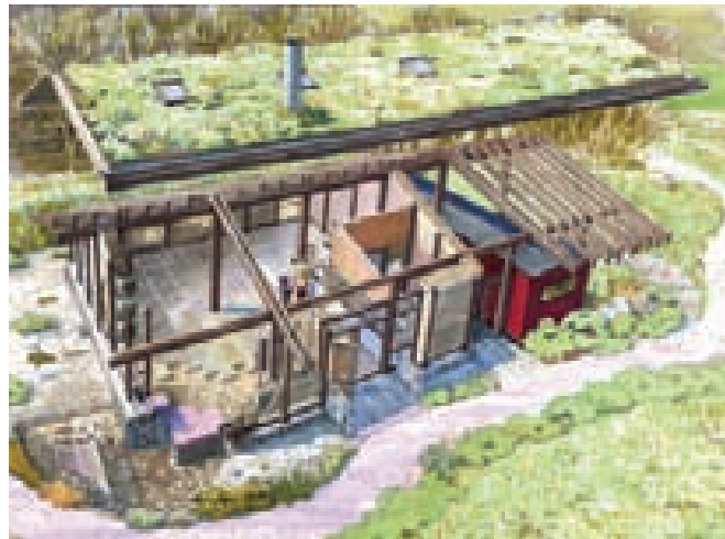
Using natural and local materials. Straw bale construction provides high thermal insulation on an exposed site with a tight budget. Very little energy was used in its construction. (Romney Marsh Visitor Centre, New Romney)
