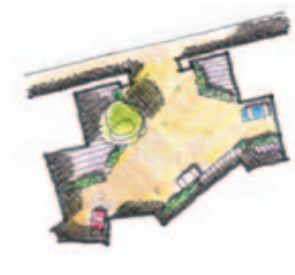
Above: A private shared access in a village setting using boundary walls to mark a line between public and private space. Left: A diagram showing a shared access to a cluster of properties in an informal layout.
