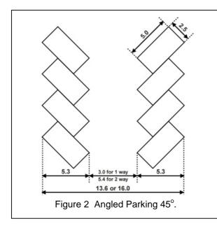
B13. Angled parking (see Figures 2, 3 & 4) is best used in car parks with one-way aisles. This enables a reduction in the width of aisles required to gain access to the parking bays. Manoeuvring into and out of the parking bays should be made easier, although with two-way aisles this may require reversing into the bays.
