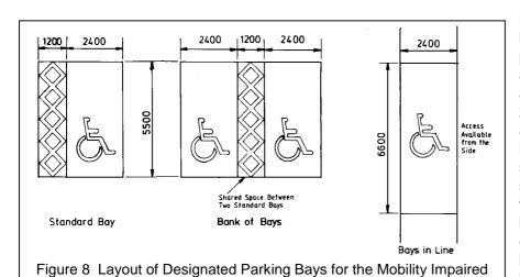
B36. Off-street parking that bays are perpendicular to the access aisle should be at least 5.5m long and 2.4m wide with additional width of at least 1.2m along one side. This should allow width sufficient wheelchair access between vehicles and enable vehicle doors to be fully opened. Where bays are adjacent to
