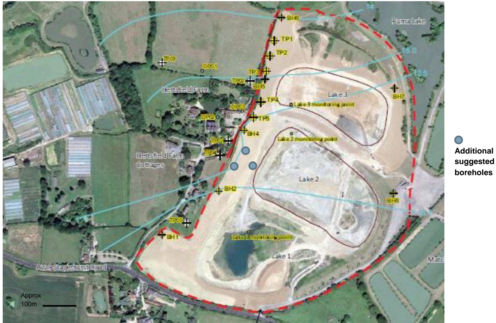
Figure 4.3: Monk Lakes site with suggested additional borehole locations
