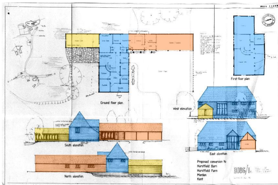
Figure 22: Morphological drawings showing the dating of the three main parts of the barn.
