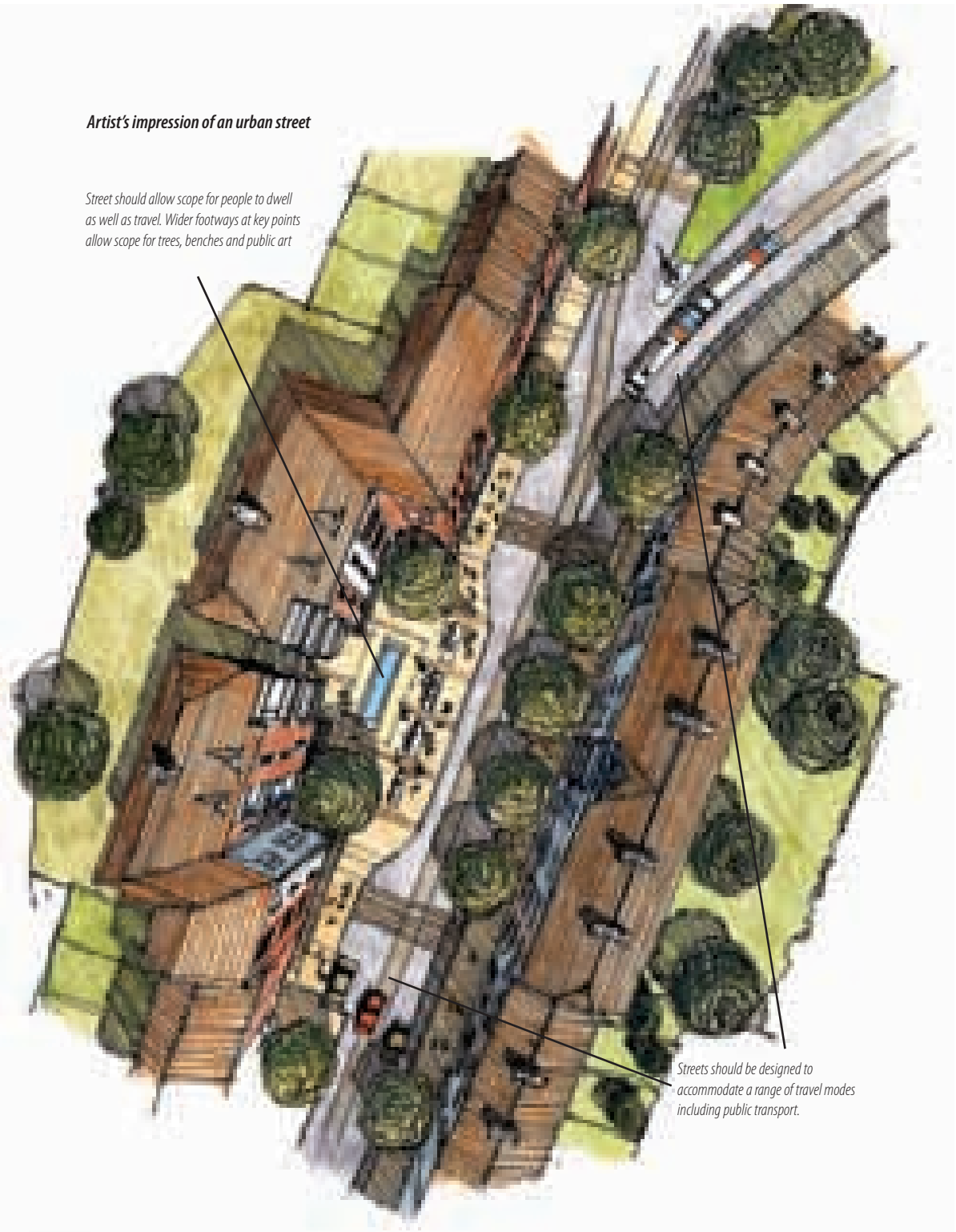
Artists impression of an urban street where residential and commercial uses are mixed. The scale provides a strong sense of enclosure. Active frontages and building entrances at ground floor open directly onto footways.
